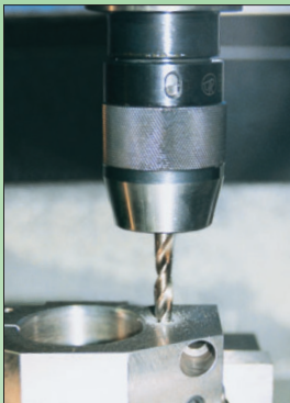
1 Drill coolant passage, leaving reaming allowance.
